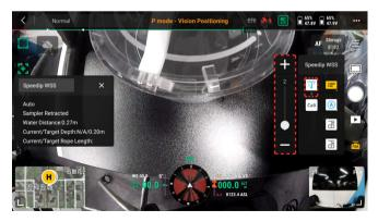
[6] Click to calibrate the rope length, the calibration function can only be used when Speedip V2 is the stationary state. Clicking the button will retract the rope and reset the length of the resealed rope to zero. Do not carry out other operations during calibration. Clicking the calibrate button again will lead to calibration failure. The calibration function cannot work when Speedip V2 is in the operational state.
