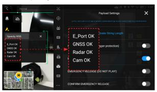
[10] Emergency Cutting Mechanism: Click on the first switch button, and the floating window will flash a prompt; click on the second switch button and it will trigger the emergency cutting mechanism of Speedip V2. Once the function is triggered, Speedip will fuse the rope within 10s, and the function will be automatically turned off within 15s to avoid damage to the internal structure due to long-term heating.
